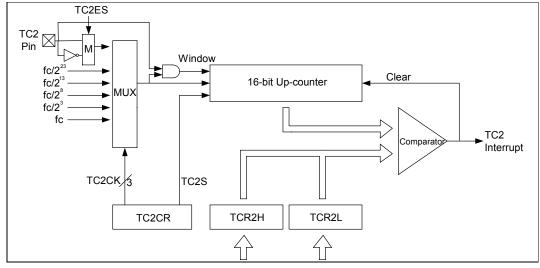
Fig. 5-18 Configuration of Timer/Counter 2
